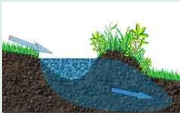
Figure 3: Swales are essentially ditches on the contour. The soil excavated to make the ditch is mounded up on the lower edge of the swale to prevent water from running over the lip. Water then percolates into the soil or can be diverted to ponds or storage.
