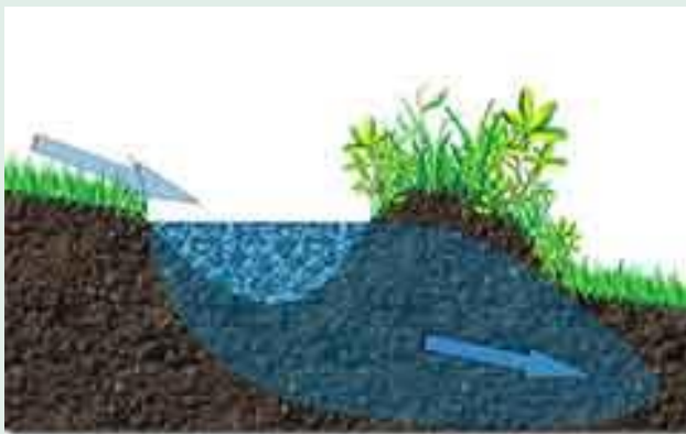
Figure 4: Swales are essentially ditches on the contour. The soil excavated to make the ditch is mounded up on the lower edge of the swale to prevent water from running over the lip. Water then percolates into the soil or can be diverted to ponds or storage.
